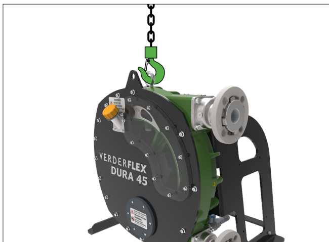
Figure 1. - Fastening Lifting Gear to Pump
