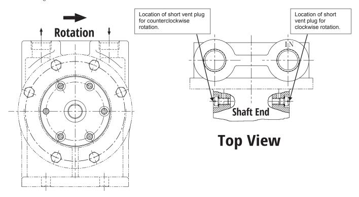
If outfitted with an internal relief valve (model CK1BV), the rotation cannot be changed in the field unless the cover/valve assembly is also replaced. To change the location of the suction port on pumps supplied with Tuthill's unique automatic reversing feature (model RCK1B), the following must be done in addition to the steps above.
