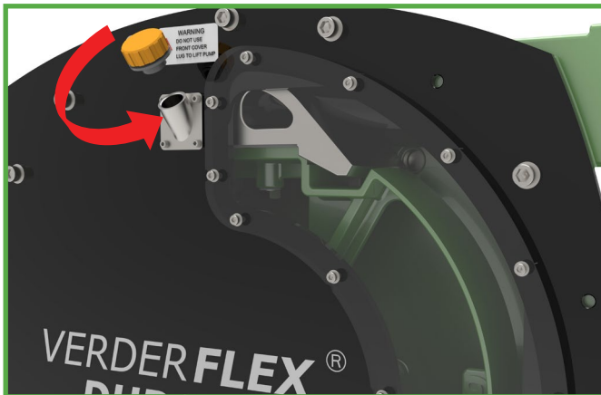
Figure 12 Filling the Pump with Lubricant
