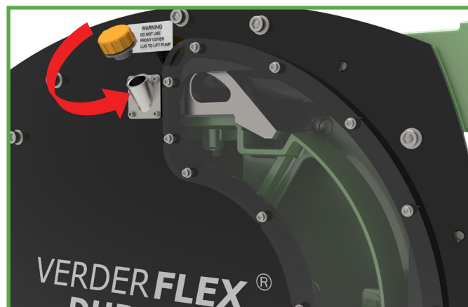
Figure 19 Filling the Pump with Lubricant
