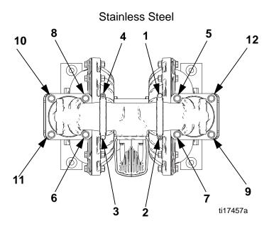
Fig. 6. Torque Instructions - Manifold Fasteners
