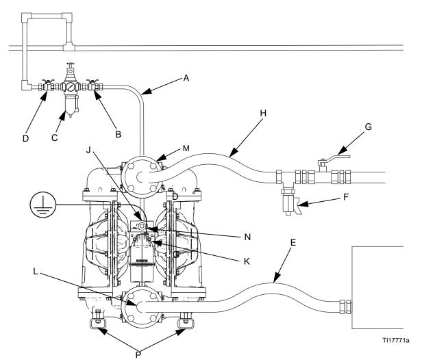
Fig. 1. Typical Installation (aluminum pump shown)
