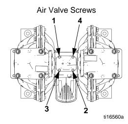
Fig. 5. Torque instructions, Fluid Covers and Air Valve Fasteners (all models, aluminum shown)
