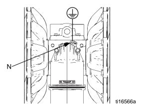
Fig. 3. Grounding screw and wire
