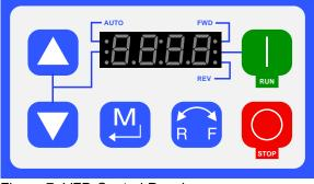
Figure 7 VFD Control Panel
