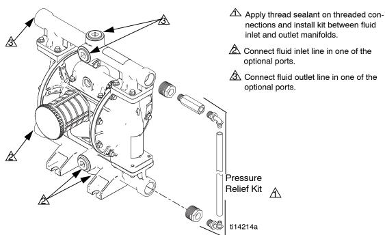
FIG. 5. Optional Fluid Pressure Relief Kit 819.6479, for Model 850.0780
