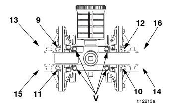
FIG. 6. Torque sequence
