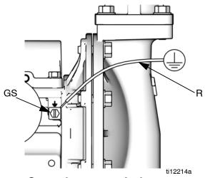
FIG. 1. Ground screw and wire
