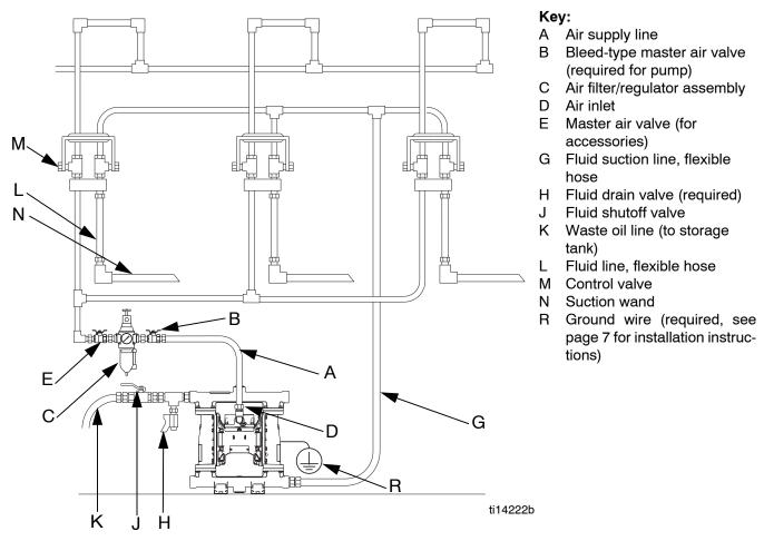
FIG. 4. Gear oil evacuation, typical installation
