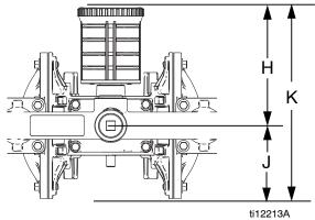
A ..... 12.7 in. (323 mm) B ..... 14.4 in. (366 mm) C ..... 15.9 in. (404 mm) D ..... 10.9 in. (277 mm) E..... 1.8 in. (46 mm) F..... 7.3 in. (185 mm) G ..... 14.7 in. (373 mm) H ..... 6.1 in. (155 mm) J ..... 3.9 in. (99 mm)
