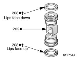
Fig. 2. Air valve u-cup installation
