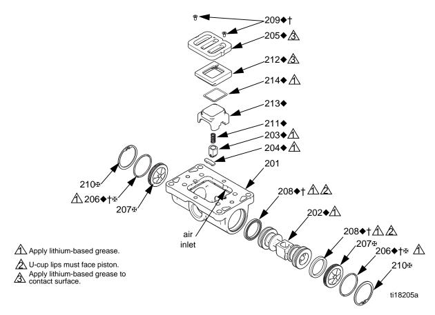
Fig. 3. Air valve assembly
