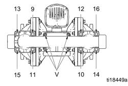
Fig. 9. Torque sequence
