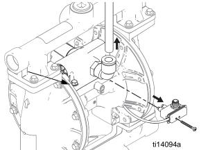
Fig. 1. Reed switch assembly and air line removal
