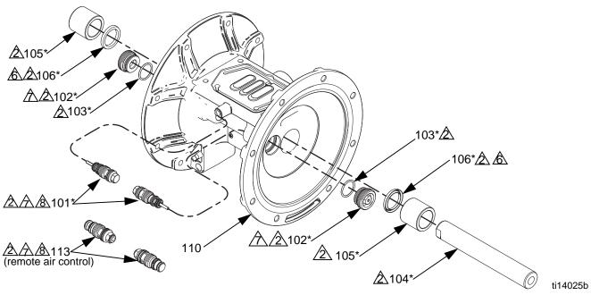
Fig. 7. Assemble diaphragms and center section
