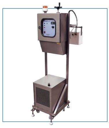
The versatile 500mm long induction coil provided as standard is designed to seal containers in the range of 20mm through to 110 mm of varying design without change. The coil mounting is fully adjustable allowing for the levelling of the head to the conveyor in both planes and the 'skewing' of the coil to maximise exposure where necessary for larger containers. Relco also manufacture custom built sealing heads and 'tunnel coils' for particular applications and unusual closure designs.
